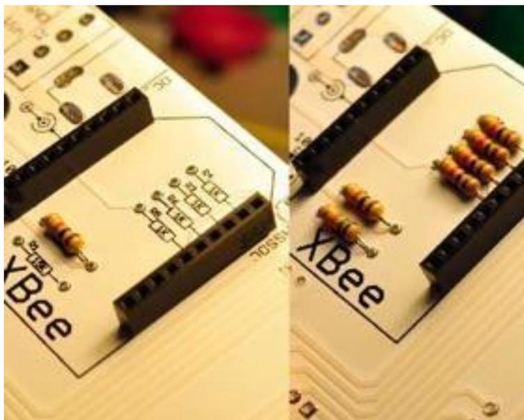
Find the 6 resistors included in kit, bend the pins of the resistor at 90 degree
