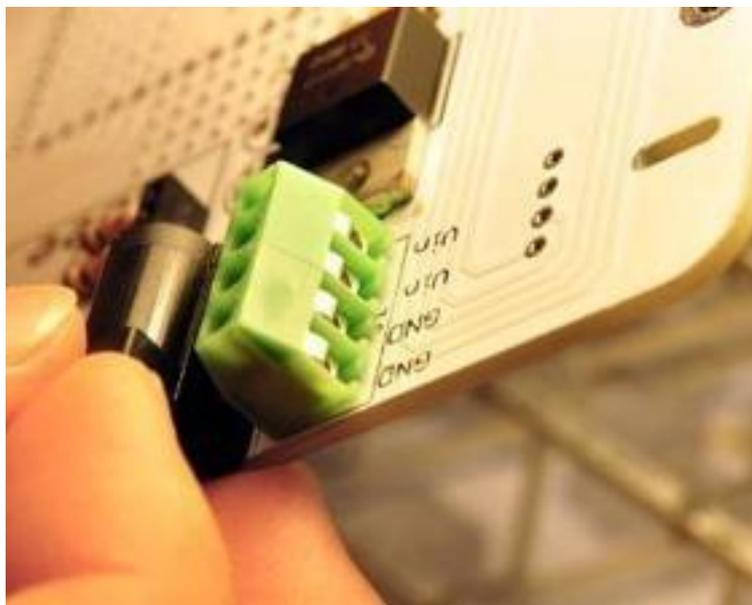
Solder the Terminal into the space labeled J1, the metal pins should line up the silk screen.
