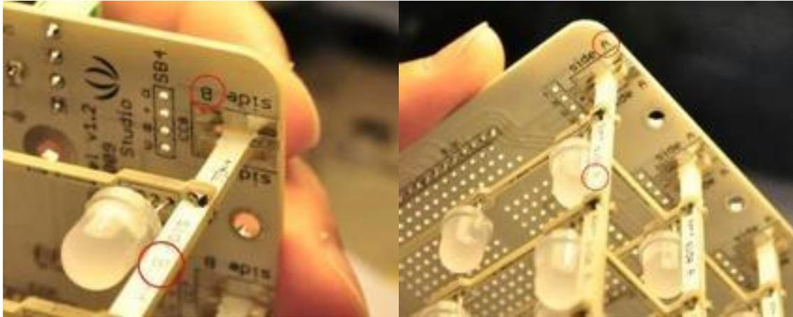
Now we should have 1 X assembled cube panel and 1 X assembled rainbow cube. Simply connect and solder them. You will find the corresponding silk screen on each board,
