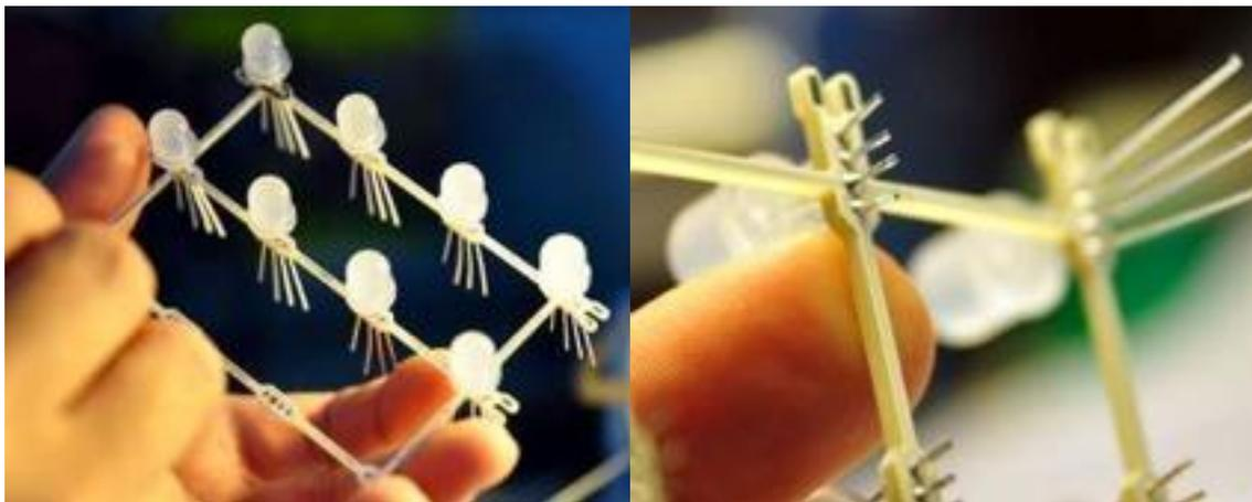
Repeat doing this, fill all 4 slim panel PCBs with LEDs, solder them and clip off the extra wires.
