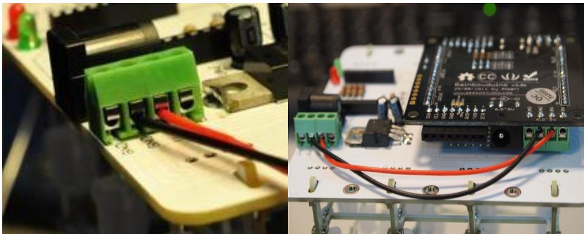
The cube is now successfully built! Before light it up, we need to connect the power cable to the terminal and connect the cable to Rainbowduino.
