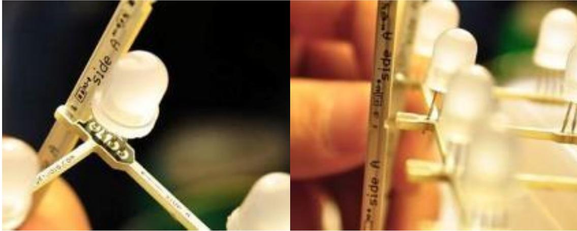
In this part we need the Side A slim PCBs. (PCB in stick shape marked Side A). Now we need to solder it to the Slim panel PCB. There's 4 of each, pick-up one randomly and find the 'Side A' silk screen and notch on both PCBs, connect them with the north and solder them together. please notice the angle needs to be at 90 degree.
