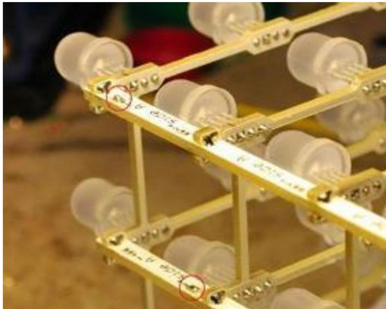
To make this cube work correctly, we need to solder 8 jumper pads on Side A and B slim PCBs.
