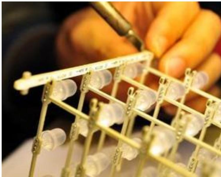
In this part we will solder 4 side B slim PCBs to the cube, pickup one randomly, find the Side B silk screen and the north on both PCBs. Connect them with the notch and solder them together. Please note that the 'side B' silk screen on Slim Panel PCBs look a bit like 'Side R', we will try fix this problem in the next version.
