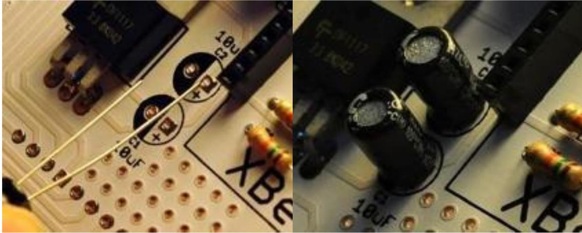
Insert 2 capacitor to the space labeled C1 C2, the longer pin should line up the square hole. Flip the PCB, solder them and trim the excess pins.
