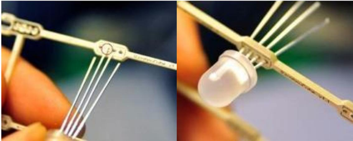
Find the bag included 70 RGB LEDs and 4 Slim Panel PCBs, hold one LED, lines up the pins and push it in. The longest pin of LED needs to line up to the square though hole on PCB,(Marked red). Notice the flat spots about 5mm away from the LED, stop pushing the LED in when the flat spots reached the PCB. Please note that the LED pins need to line up to silk screen.
