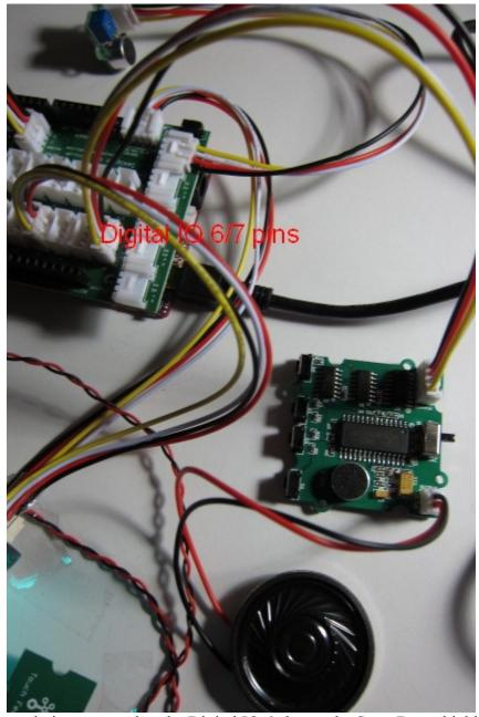
The sound recorder twig is connected to the Digital IO 6 slot on the Stem Base shield.
