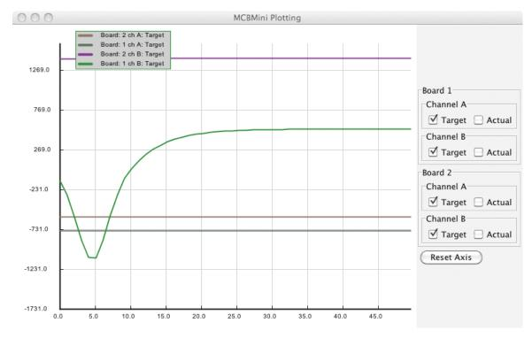
In this window the user can observe target and actual values for all the controllers. This is often crucial to tune the controllers for different setups.
