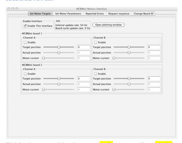
This is the main motor target window where a user can specify motor target positions or velocities and observe instantaneous feedback values.
