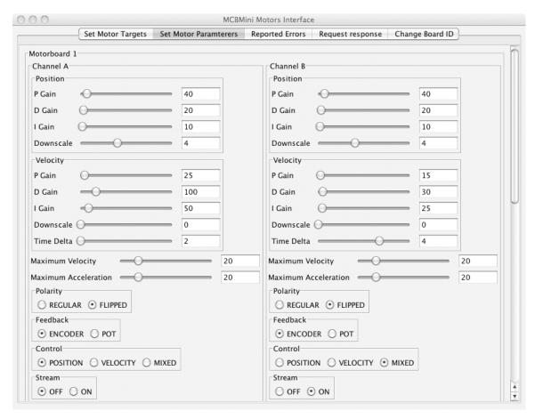
In this window the user can specify various parameters for the boards and change them on the fly. These parameters are read from a configuration XML file.
