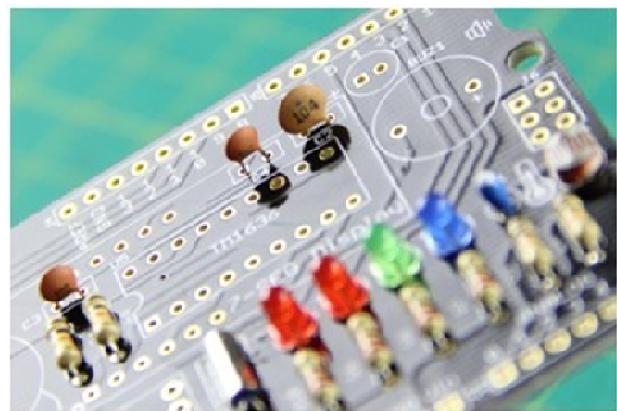
For the square black capacitor, make sure the longer lead goes in the hole marked with a "+". This is very important as capacitors are polarized just like the LEDs.
