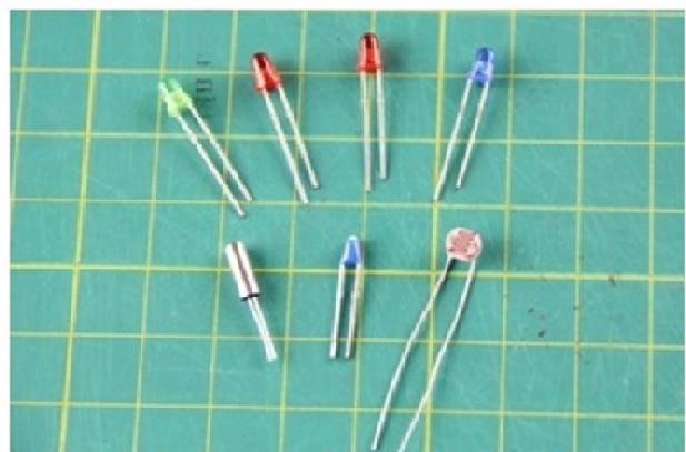
In the second row, from left to right, are a crystal, a thermistor and a light dependent resistor. They are not polarized, meaning it doesn't matter which way they are inserted into the board.
