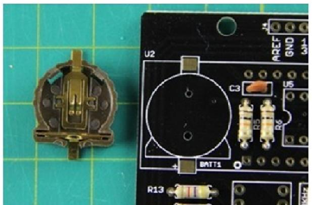
This is the only surface mount component in this kit. Surface mount just means the component is soldered onto the surface of the board as opposed to through hole like the other components. Soldering it is very similar to soldering the crystal to the pad.
