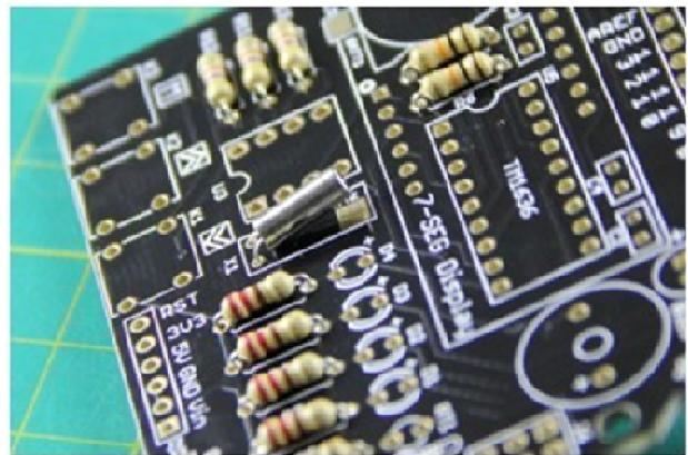
There is a square locating pad on the board that helps you keep the crystal flush. Melt some solder on the pad first.
