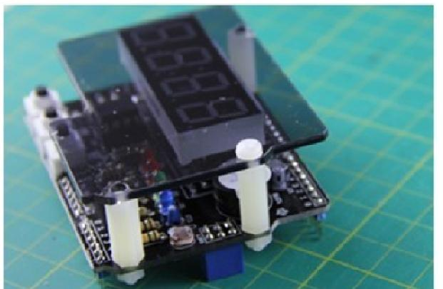
Tighten the standoffs with screws from the top.
