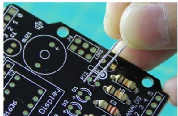
Just like the resistors, the thermistor and light dependent resistor are not polarized so it doesn't matter which way they are inserted, simply insert both leads into the board.
