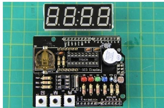
Insert the U3, U4 and U5 chips into their locations by snapping them into the IC sockets. It's very important to align the chips per the half-moon shape on the chip to the half-moon shape on the board.
