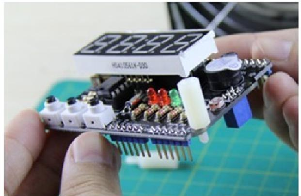
From below, secure the standoffs to the board, by screwing a nut onto each one.
