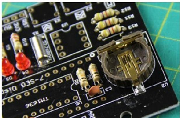
Now let's move on to the sockets. Search for the half-moon shape on the board. This is the directional indicator for the IC Sockets. It is very important that the orientation of the IC socket is correct. After soldering the 4 LEDs and 2 sensors, the board should look like this:
