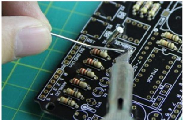
Now push down the crystal and add more solder to the locating pad. When cool, the crystal should stick to the pad.
