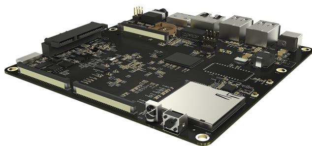
LOFT-Q is the second prototyping board of Mixtile project. Based on AllWinner A31 SOC, designed for embedded developers, engineers, makers and hackers, it can be used as home media center, personal could device, NAS, etc. This guide will help developers quickly building the environment, compiling usable os and customizing you own application.
